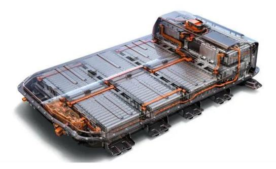
333. The Bolt's battery is structured with the cells<sup>62</sup> arranged "like books on a bookshelf, in groups." Each group of pouch cells is "stacked to make modules," which are "held together at the ends by long bolts." The [battery] pack thermal management is regulated by sensing temperature via thermistors located at the ends of the modules" and the liquid coolant is distributed via channels at the base of the cell packs. 65
